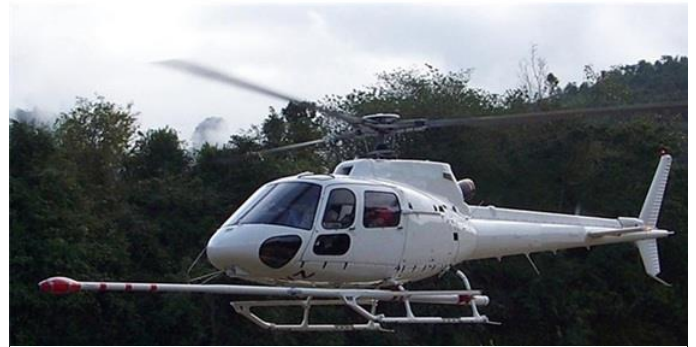
HELIMAG&SPEC “stinger” system installed on an AS350B2 helicopter. The gamma-ray spectrometer system is installed in the helicopter cabin
