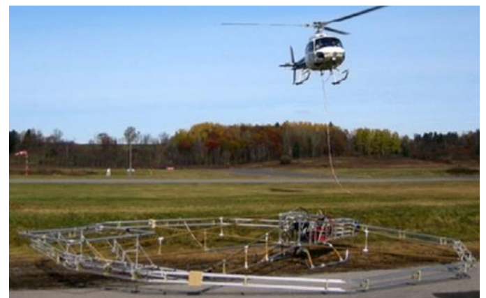
THEM multi-sensor system with time domain EM, magnetic & gamma-ray spectrometer sensors typically installed on an AS350B2 or B3 helicopter
