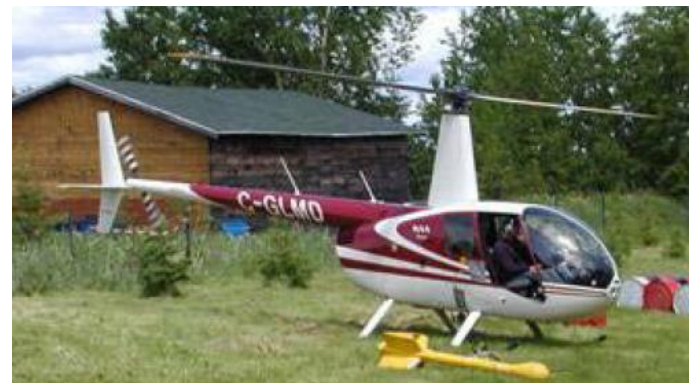
HELIMAG towed-bird magnetometer system installed on a Robinson R44 Raven helicopter.
