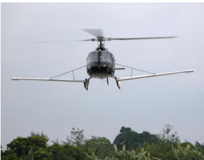
HELIGRAD magnetic gradiometer with 2 magnetometer sensors and gamma-ray spectrometer installed on an AS350B2 helicopter.
