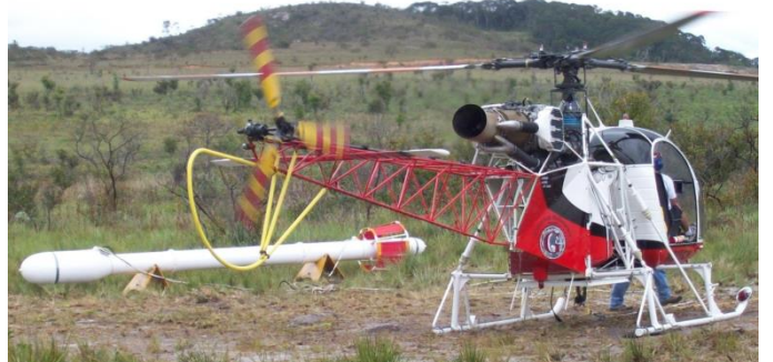
HUMMINGBIRD multi-sensor system with 5-frequency EM, magnetometer & gamma-ray spectrometer sensors installed on a AS315B LAMA helicopter.
