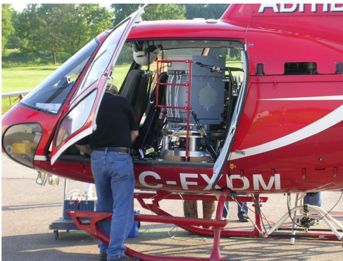
HELIGRAV with GT-2A airborne gravity sensor and magnetometer & GPS navigation.
